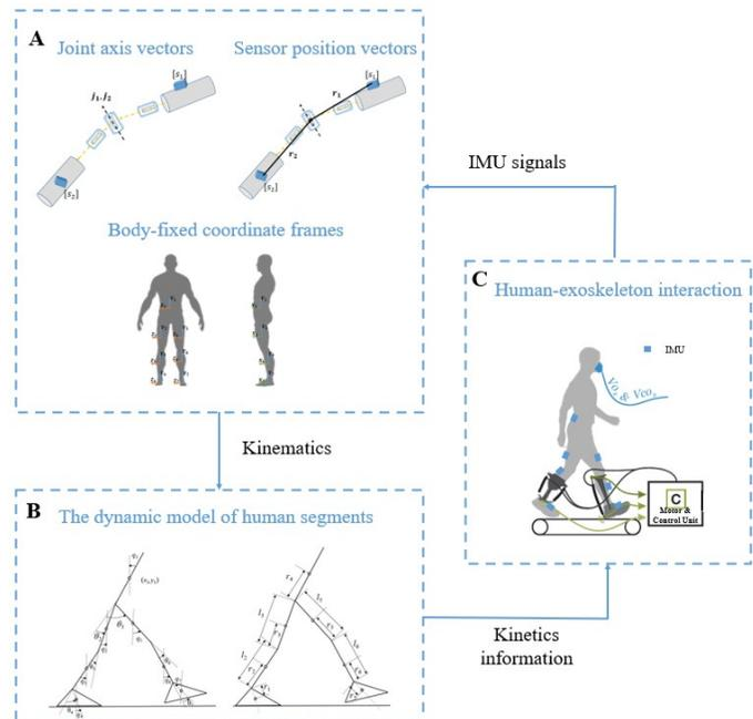
Fig. 1. A schematic diagram of the information flow. (A) Kinematics calculation. (B) Kinetics calculation. (C) The diagram of sensing signals from human and applying calculated kinetics to controlling exoskeletons..
